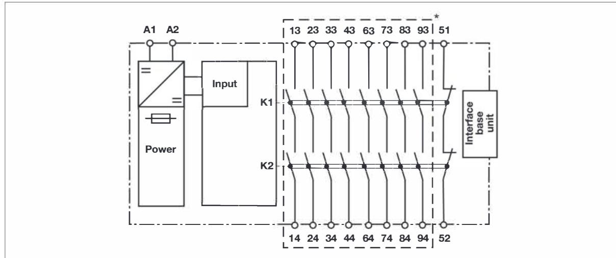
\*Safe separation in accordance with EN 60947-1, 6 kV
